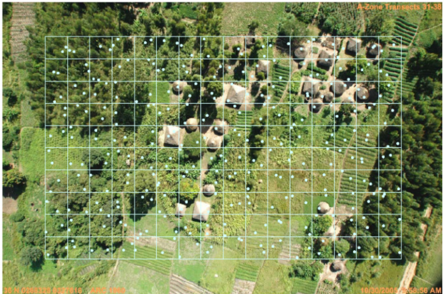
Figure 3.1. The dot-grid used for the analysis, over a scene from Arua. The surface area covered by the frame is a function of the flight height, which is monitored during flight. For the Arua interpretation, the calibration between the aircraft radar altimeter and photogrammetry gives a mean airphoto area of 4.18 ha, with a central interpretation area within the 320-dot grid of 2.57 ha.
